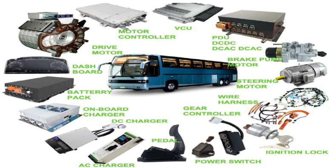
Figure 5.17.1: EV Converted Bus
